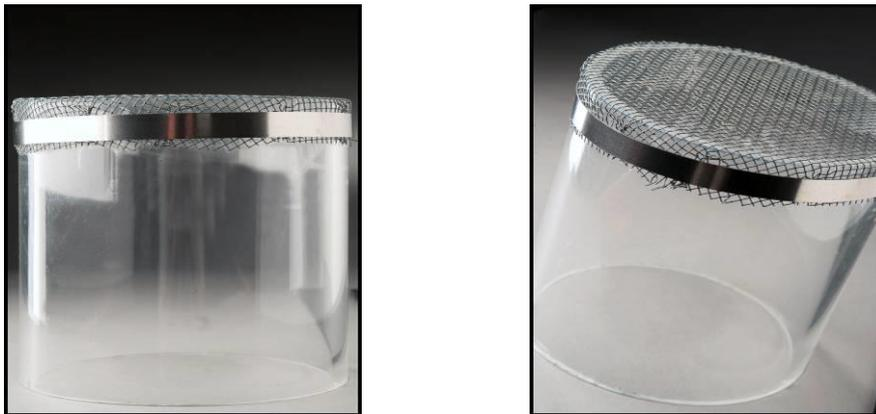
**Figure 3.** Cup-like device used to assess Holding impulse. Left side shows cup upside down (bottom of cup at top) and right side shows the cup bottom tilted to expose the aluminum mesh screen. The mouse is placed upright on the mesh screen inside the cup before the cup is turned upside down.
